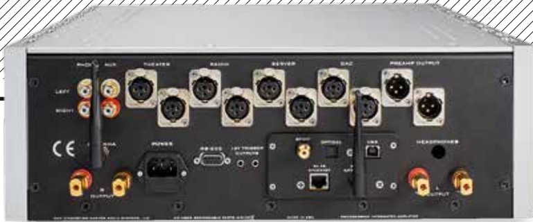
ABOVE: Fully loaded, the amp offers four balanced line ins on XLRs, one MC phono and a line in on RCAs. Antenna [left] is for the BT remote, the other for wireless Wi-Fi alongside Ethernet, USB-B, coaxial and optical digital ins. Outputs include 4mm speaker binding posts, one balanced pre out (on XLRs) and a 6.35mm headphone out
